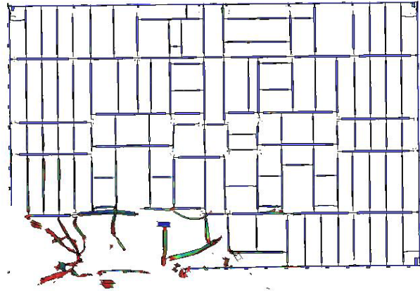
(b) Floor 81 core framing damage
