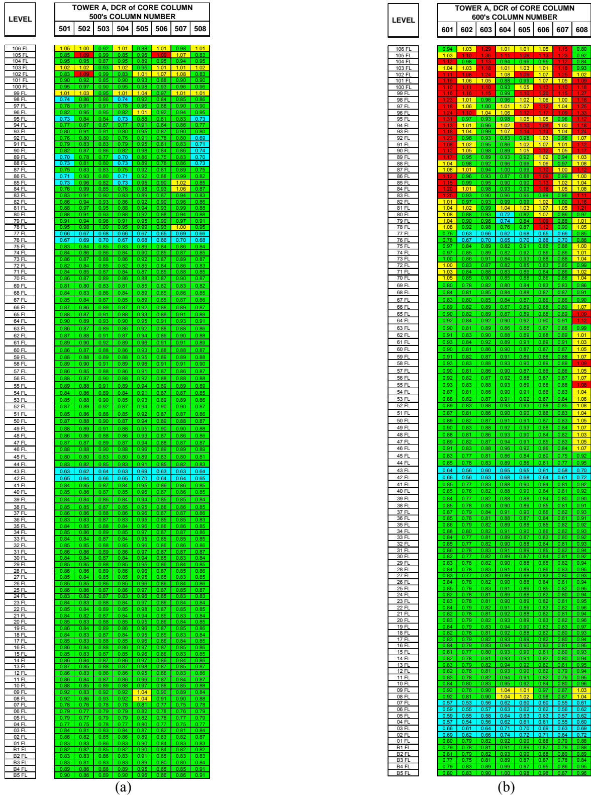
Figure 4-5. DCRs for WTC 1 core columns under original design loads, (a) 500 line, and (b) 600 line.
