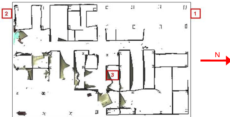
Figure 7–77. Base case stairwell disruption on floor 78 in WTC 2.
