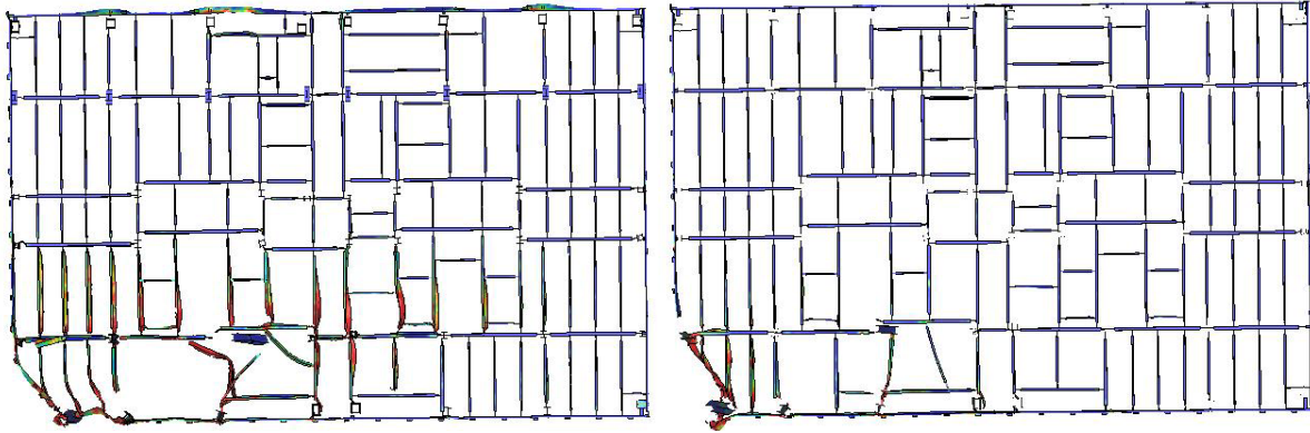
(a) Floor 80 core framing damage (b) Floor 81 core framing damage Figure E-48. Base case impact damage to the core beams of floors 80 and 81 of WTC 2.
