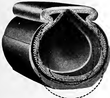
U SHAPED TIRE UNDER LOAD
