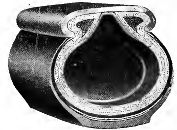
RAISED TREAD OVAL TIRE NATURAL SHAPE UNDER LOAD
