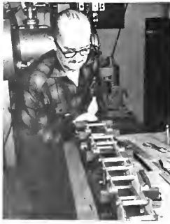
A workman at the General Electric Atomic Plant Equipment Department in San Jose, California, fabricates fuel elements for the Vallecitos Atomic Power Plant.
