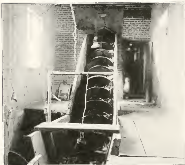
THE "SCROLL" OR WORM CONVEYOR WHICH LIFTS THE BEETS FROM FLUME INTO FACTORY
