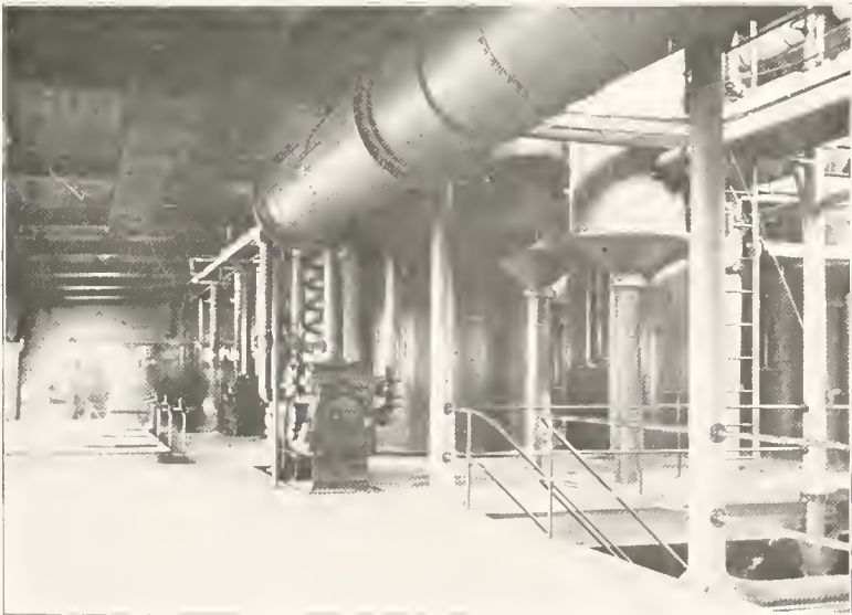
SYRUP BOILERS, OR "STRIKE PANS," IN WHICH THE RICH SYRUP IS CRYSTALLIZED TO SUGAR
