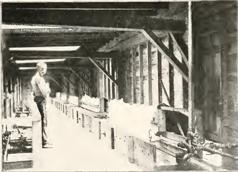
AUTOMATIC RAKES DUMPING SALT FROM GRAINERS ONTO CONVEYORS SAGINAW PLATE GLASS COMPANY
