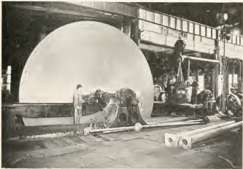
PIT LATHE IN BARTLETT PLANT FINISHING OFF "DECK" FOR SAGINAW PLATE GLASS COMPANY
