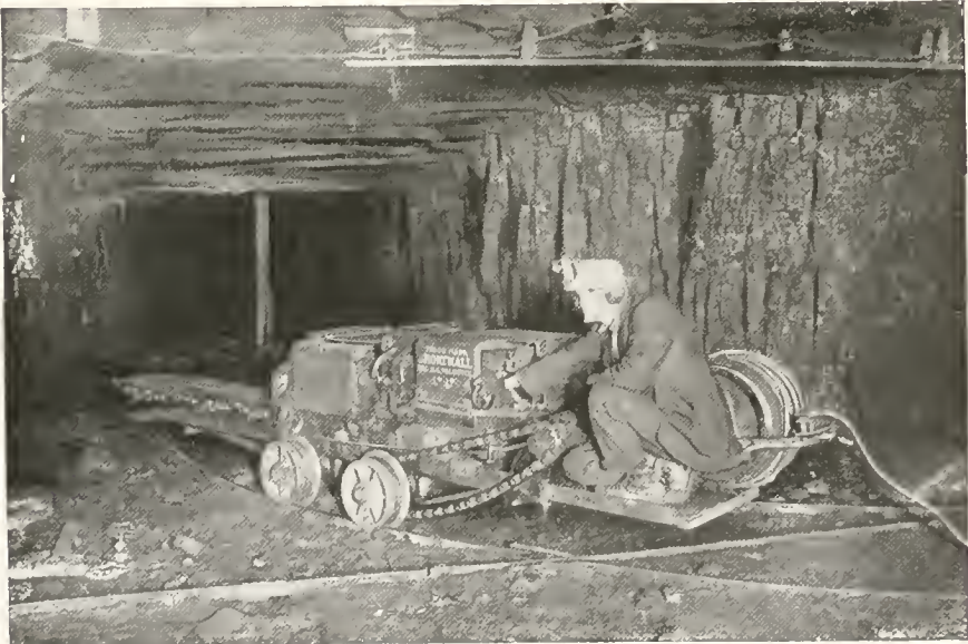
ELECTRIC CHAIN CUTTER OPERATING IN ENTRY
