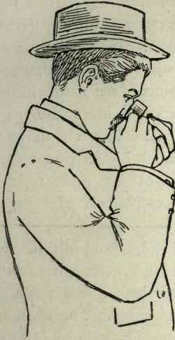
Correct manner of holding magnifier and object.
