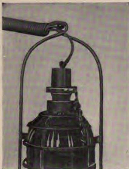
FIG. 5.—Collecting Bottle Showing Stopper with Upper Part in Place. After Eurich.
