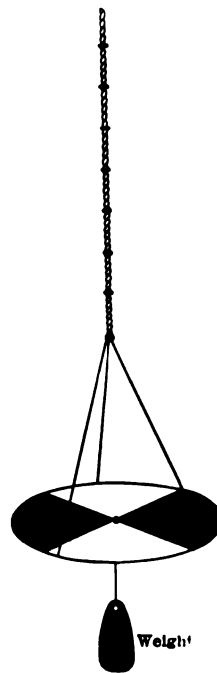
FIG. 48.—Disk for Comparing the Transparencies of the Water in Different Lakes.
