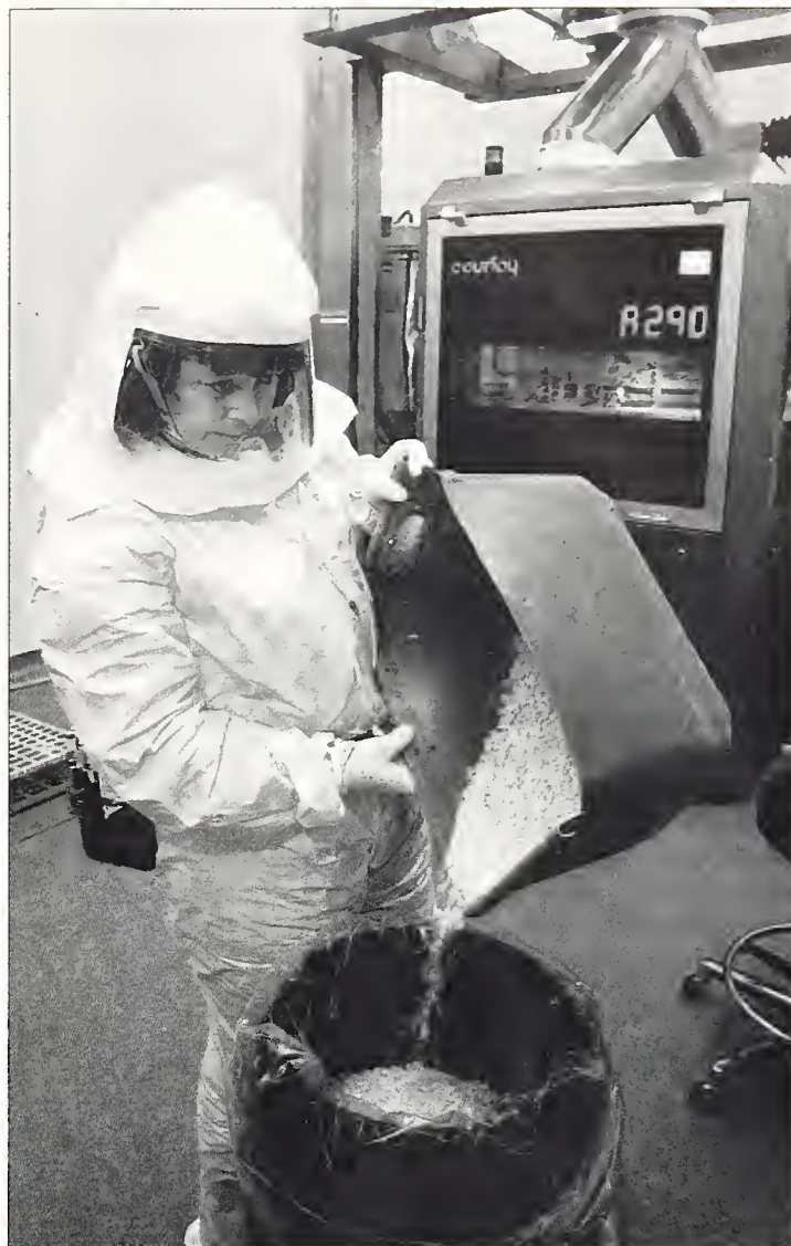
Fig 1: The medical history of chemical workers should include information on whether personal protective equipment was used. Here, a manufacturing operator at Glaxo, Inc., prepares pressed tablets for transport to tablet coaters at Glaxo's manufacturing and packaging facility in Zebulon. Photo courtesy of Glaxo, Inc.
