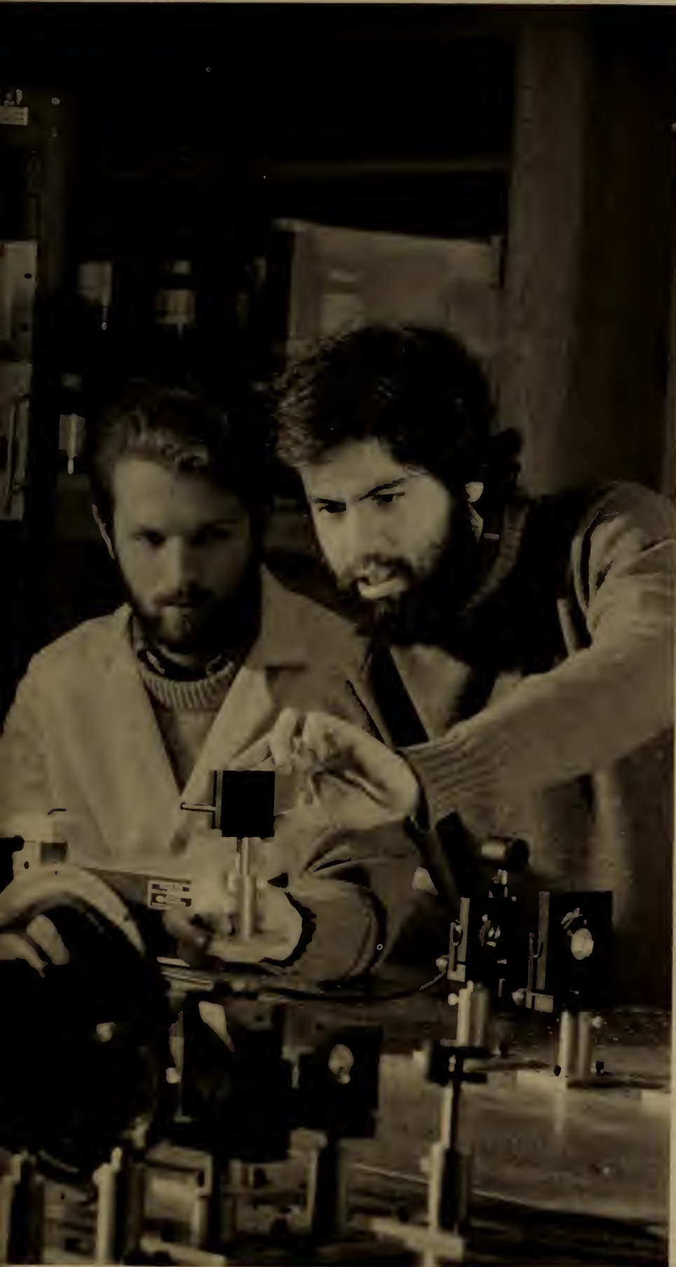
Prof. David Statman (right) demonstrates for student James Shea the alignment of optical components for picosecond spectroscopy.
