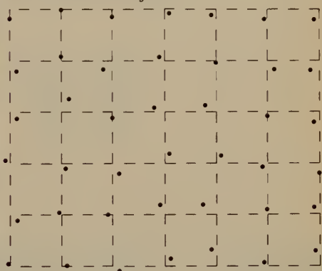
Figure 2. Nonperiodic, or amorphous, structure. The atoms are placed in random positions and the distance between them is no longer d .
