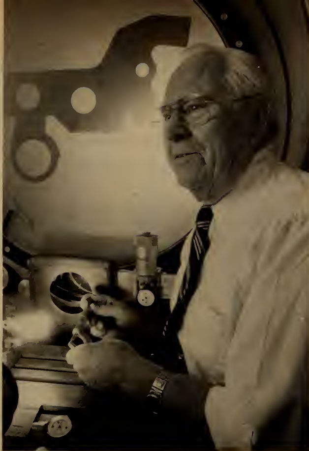
Gustafson at Lundquist's optical comparator, which magnifies fabricated parts to enable testing of sphericity and linear dimensions.
