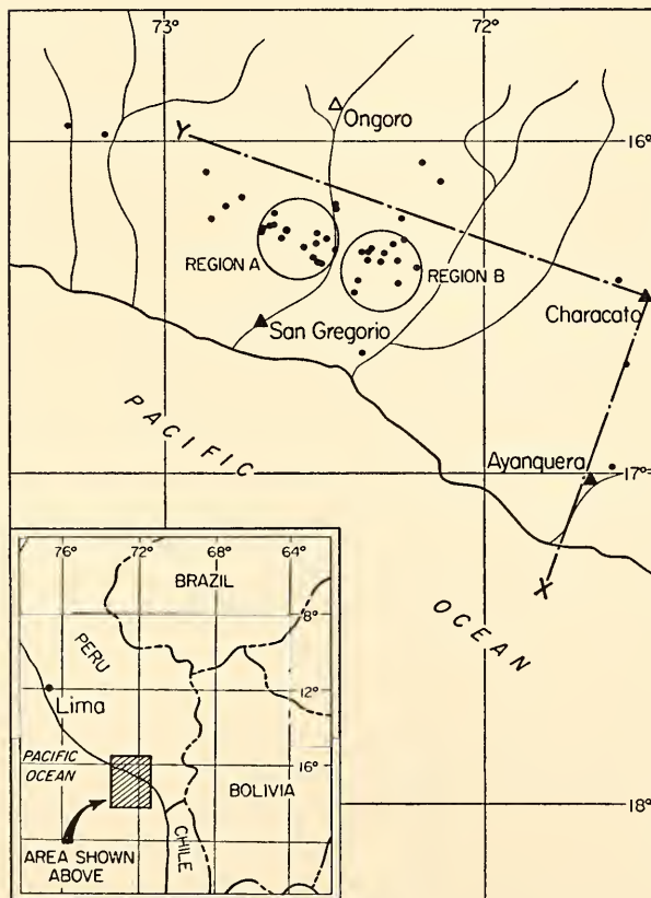
Fig. 15. Arequipa, Peru, seismic network. Regions A and B (encircled) designate where numerous local earthquakes have occurred, and the earthquake epicenters are shown.
